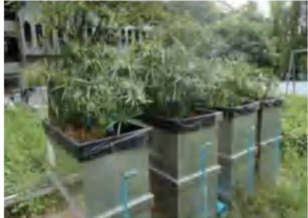
Constructed wetland using umbrella sedge plant developed by TISTR.
